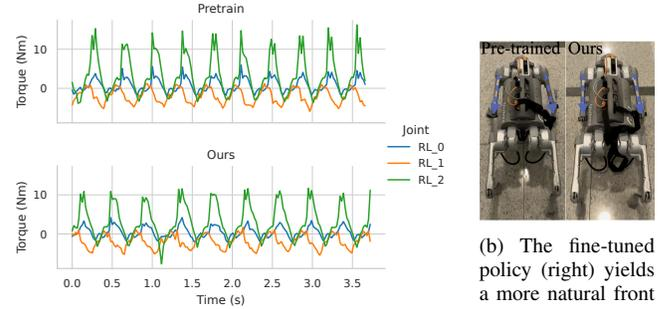
(a) Joint torque profiles of the rear-right leg for pre-trained and fine-tuned policies.
