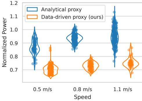
Fig. 3: Distribution of normalized net power ( $\frac{P^{\text{fine-tuned}}}{\text{Mean}(P^{\text{pre-trained}})}$ ) for the policies fine-tuned with the baseline and our framework. Each point represents a 1-second segment within the test run.
